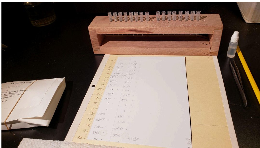
Figure 1. Setup for speed-spotting TLC plates. A numbered wooden rack holds the pipette tips loaded with lichen fragments; two overlapping labeled silica gel plates are ready for spotting. The two identical plates will be run in different solvent systems. The forceps and acetone dropper bottle are used for plucking lichen fragments and loading the tips.
